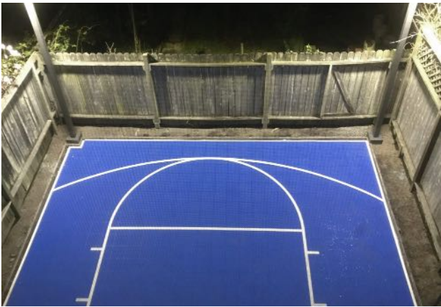
Half-court pad on two poles, spill-control optics inside a residential fence line.
