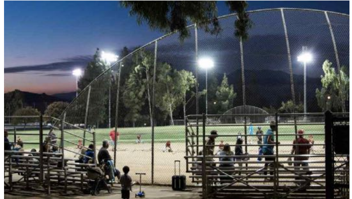
Infield and outfield carry different targets. RP-6-20 Class III asks 50 fc infield and 30 fc outfield.
